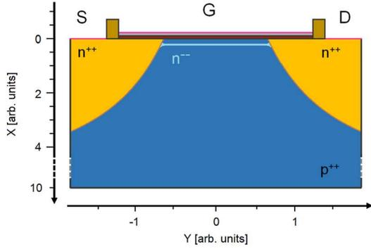
Fig. 2: Cross section of the 250 nm nMOS Bulk device with slightly n-doped buried channel implant for RTN performance improvement.
