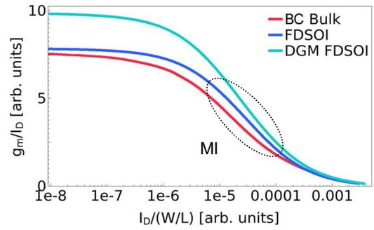
Fig. 8:  $g_m/I_D$  vs.  $I_D/(W/L)$ : In the moderate inversion regime and above the FDSOI device shows a drastically increase of the intrinsic gain  $g_m/I_D$  compared to the conventional BC Bulk device.
