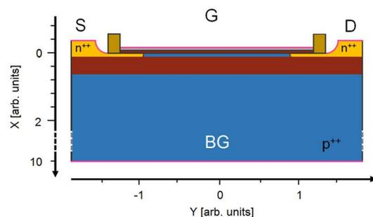
Fig. 1: Cross section of the 250 nm nMOS FDSOI device with HKMG, epitaxially grown S/D regions for lower contact resistance.
