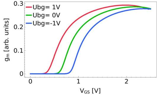
Fig. 5:  $g_m$  of the FDSOI transistor at different back gate voltages.
