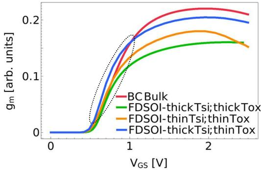
Fig. 4:  $g_m$  vs.  $V_{GS}$ : The FDSOI device shows a higher channel control at low voltage supply by combining the individual optimized layer thickness ( $V_{GS} = 0.6-1.0$  V).
