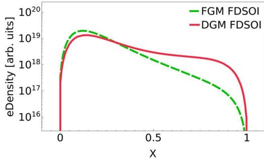
Fig. 7: Electron density distribution of the FDSOI transistor in FGM and DGM simulated at  $5\mu\text{A}$   $I_D$ . The lower electron density at the same current near the front gate of the DGM FDSOI indicates higher charge carrier mobility in comparison to the FGM FDSOI.
