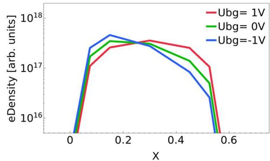
Fig. 6: Electron density distribution of the FDSOI transistor simulated at  $5\mu A$   $I_D$  with different BGM voltages.
