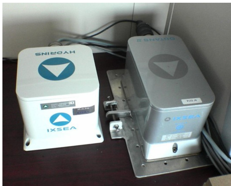
Figure 4: INS-Systems HYDRINS and OCTANS III made by iXSea (Röttger 2008)
